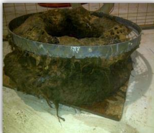
Photo 3-1 An algae clogged intake basket from a surface water treatment plant
